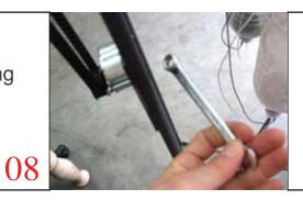
Unscrew a little the motor to make a loose tension on the belt. Remove the belt.
