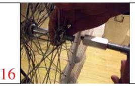
When the 2 nuts are loose, you can remove the wheel from the stand.
