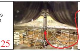
Long nut between 2 wheels. Do not force to screw too tight. When it stops, STOPS.
