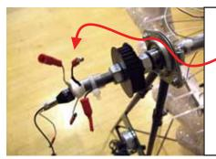
Unplug all "Slip Rings". To deconnect the red connection, you have to hold each side and twist.
