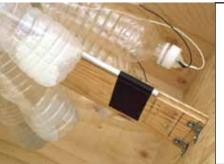
Tape the aluminum rod to the wooden support to be sure it does not move during the
