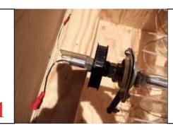
Make sure the little wires are free and the axis is protected by the transparent plastic tube. 35
